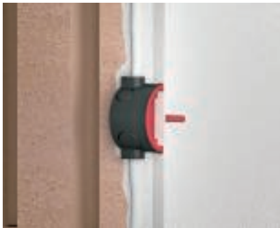
Signal cover Before plastering, place the signal cover on the device or connection sockets. They prevent soiling of the socket interior and simplify finding the sockets again after plastering.
