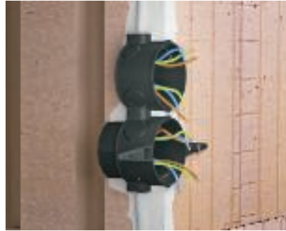
Combination of concealed sockets The accessory sockets and the device connection boxes can be interconnected using their tunnel supports. The combination spacing is 71 mm.
