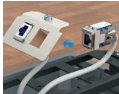
Mounting of Snap-In fastening frame Attach the Snap-In fastening frame to the connection module from the front and lock it in place. The Snap-In fastening frame allows the installation of the data technology modules in underfloor systems using a mounting support or support plate with a mounting opening 19.3 x 14.8 mm (Type C).
