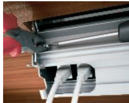
Adjustment of cover resistance The resistance or movement of the cover is adjusted using two adjusting screws on the lower side of the Deskbox.
